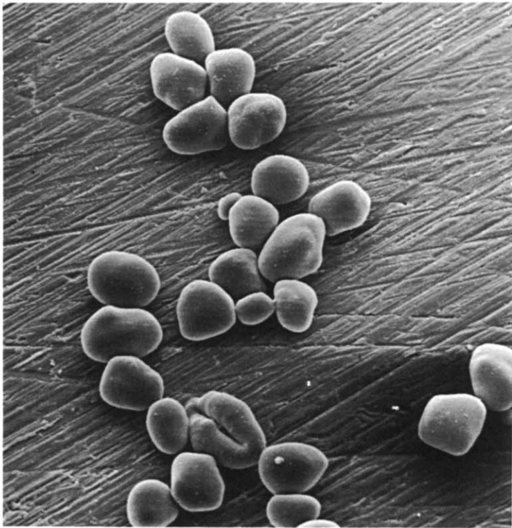
Figure 5. Starch particles of 50\ \mu\text{m} dia under the electron microscope.
